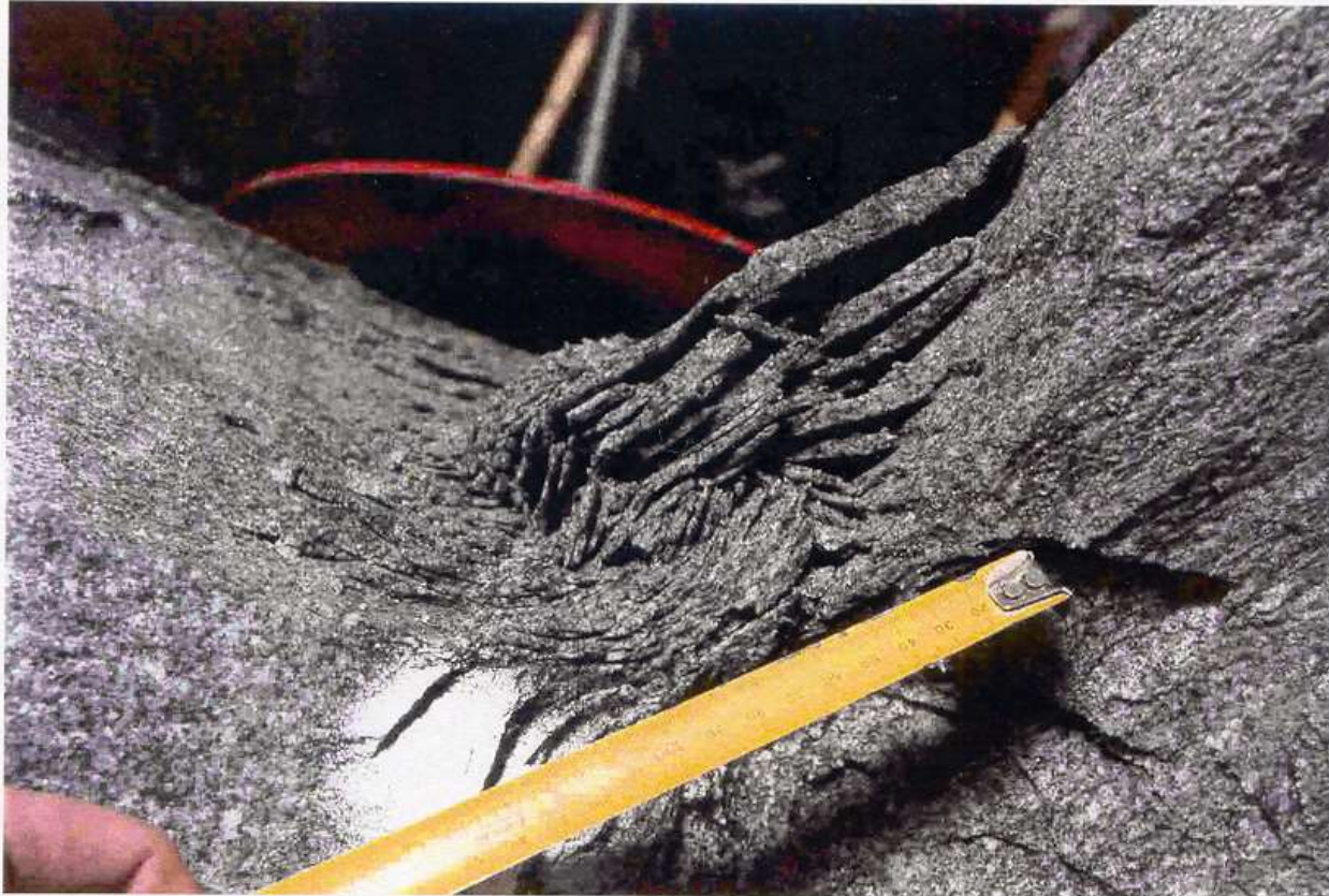
Figure 95: Close-up of the Notch Tip in the Mine-by Experiment Tunnel Showing Dilation in the Process Zone
