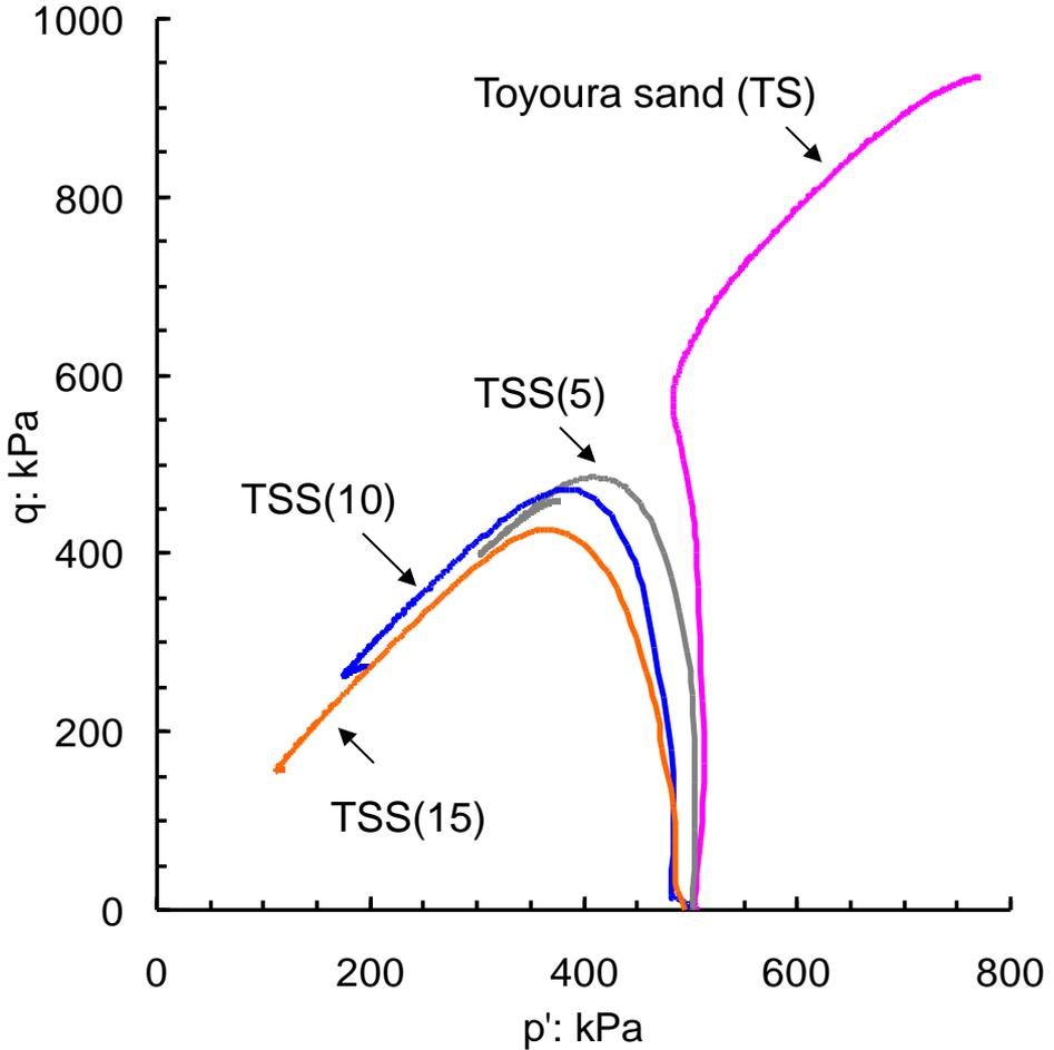
Undrained shear behavior of Toyoura sand modified by crushed silica fines
