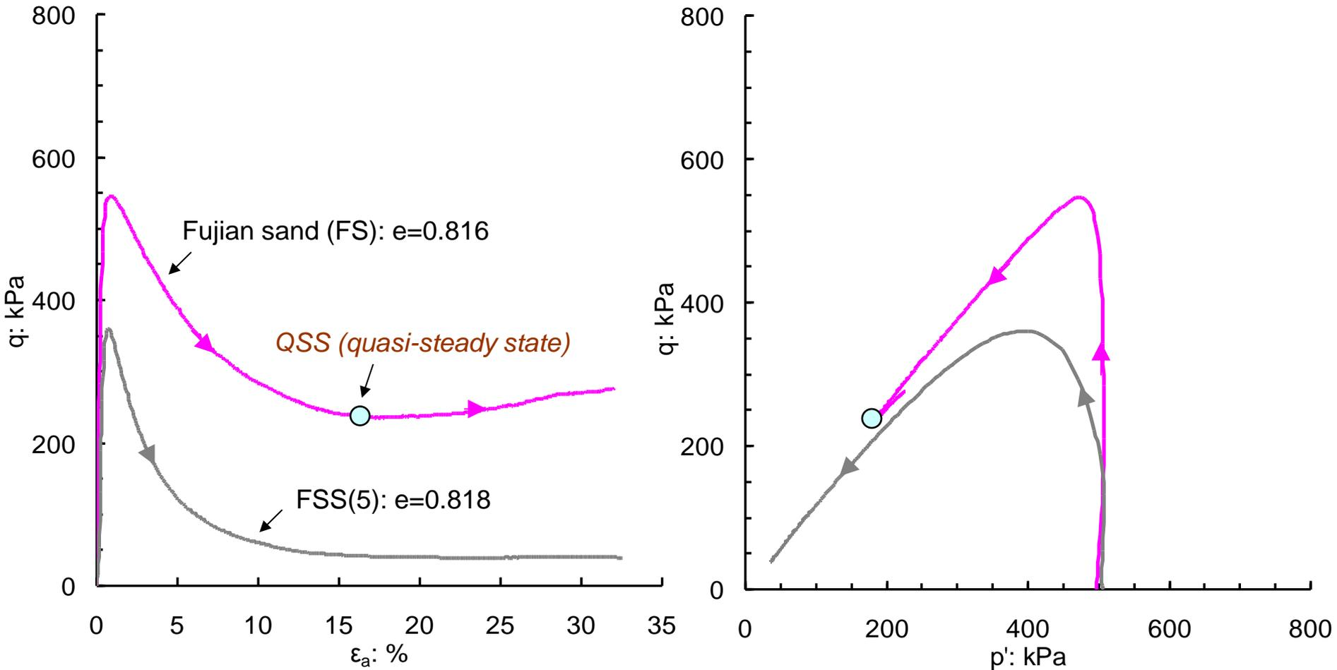
Undrained shear behavior of Fujian sand modified by crushed silica fines
