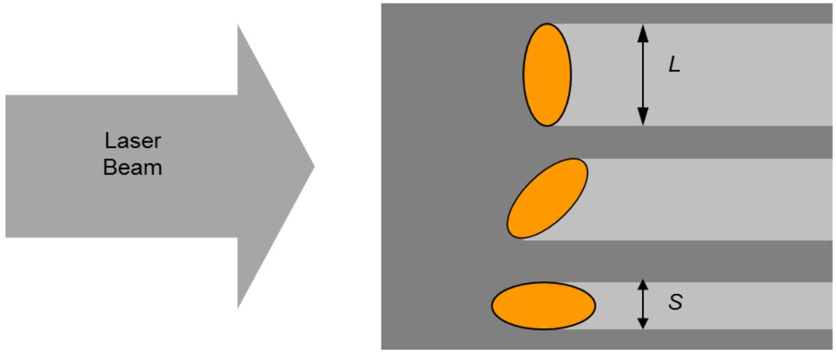
Laser Diffraction (LD) method for particle analysis
