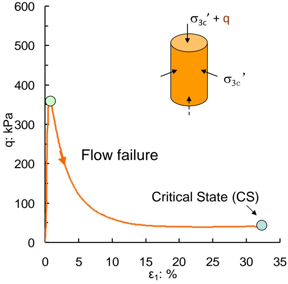
Static liquefaction or flow liquefaction is characterized by a sudden loss of strength and a rapid development of deformation in a mass of saturated granular soil. It can be triggered by either monotonic or cyclic loading and can produce the most catastrophic effects of all liquefaction-related phenomena.
