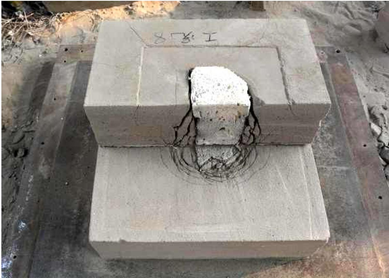
*Fig.10 Macro fracture mode of model ZD-2*
