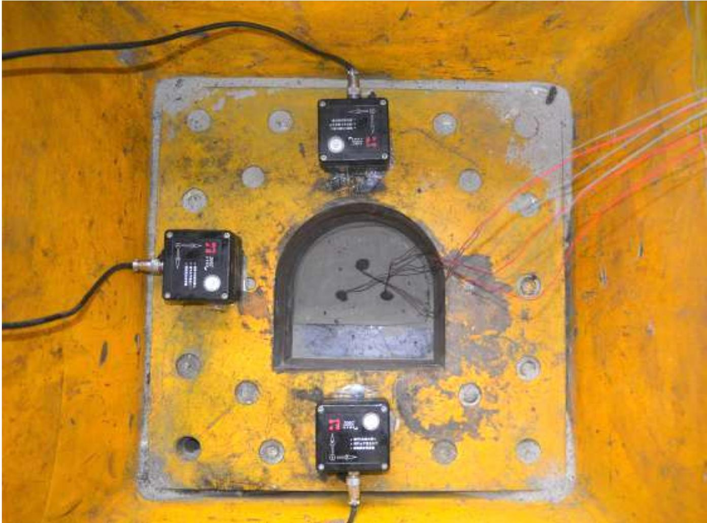
*Fig.6 Blasting excavation in 3D geomechanical model experiments*
