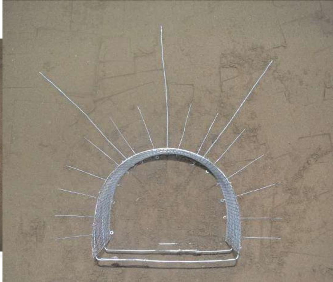
*Fig.11 Layout of model support materials
