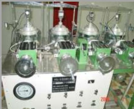
quadruple direct shear apparatus for unsaturated soil
