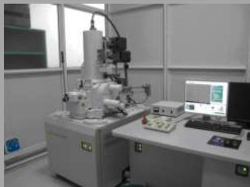
JSM-7500F scanning electron microscope
