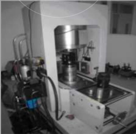
**RMT-150C rock mechanics test system**
