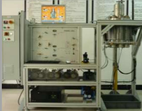
**Adaptive automatic triaxial testing machine**
