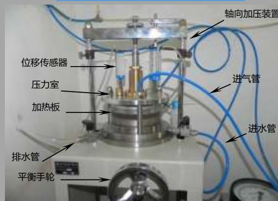
The soil-water characteristic curve tester
