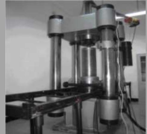
**RLW-2000 triaxial creep test system**
