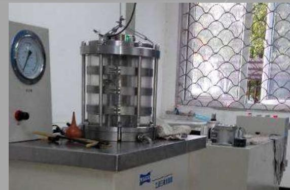
Computer controlled electro-hydraulic servo soil dynamic triaxial testing machine
