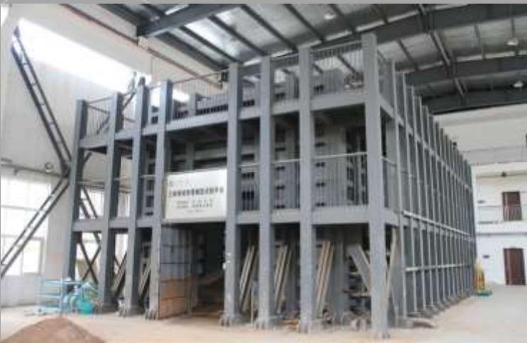
Three dimensional landslide physical model test system (12m x 6m x 6m)
