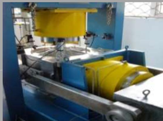
DHJ-50 large single shear direct shear apparatus
