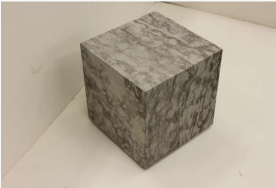
406 mm Cuboidal Sample -Surface Dry
