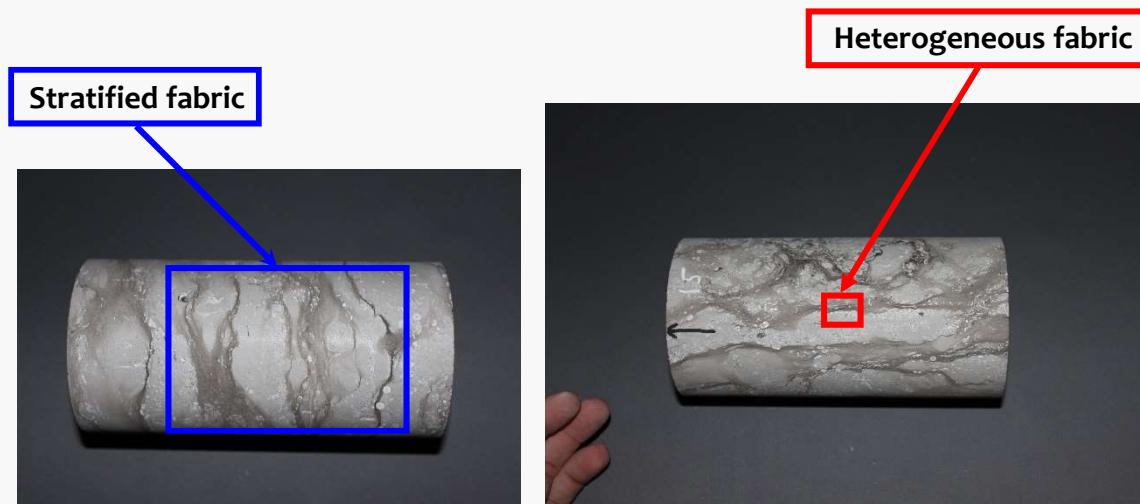
The Cobourg Limestone Cores- 85 mm diameter
