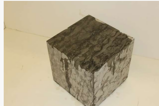
406 mm Cuboidal Sample-Surface Moist
