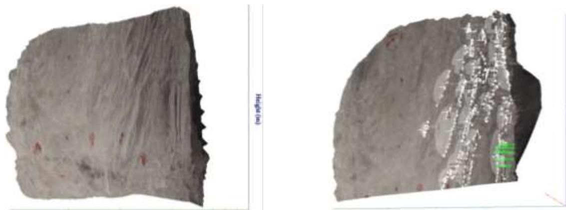
3D images of rock surfaces after identifying slabbing characteristics
